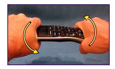
If the 'twist' results in a change of behavior, it usually is an indication of these faulty joints, most commonly underneath the processor (CPU), which is the largest chip on the board. Although this condition can sometimes be repaired by re-flowing the solder underneath the chip, this procedure is difficult, not always successful and generally not cost-effective to do.
